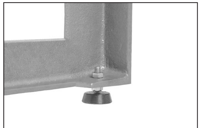
Figure 12. Machine feet installed.
